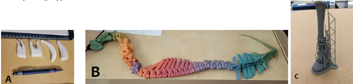
Figure 1: Example teaching tools created by 3D printing: (A) teeth, (B) spine, and (C) bones of the lower limb including the 3D printing support structure.
